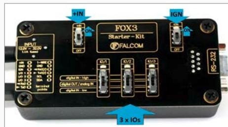
Figure 11: Top panel of the control-box.
